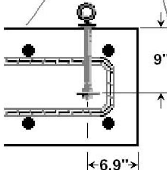
(4) 1/2" x 10" Forged Eye Bolts (2200 lbs) secure tank to weight. Galvanized eyebolts cast in place 9" deep to 3"x3" x 3/16th" foundation plate washers secured top and bottom with round washers and nuts. Eye bolts rated 2200 lbs. Tank secured to ballast by coated galvanized steel cable clamped in place at top of tank. Sacrificial anode and foundation sump pump protect the installation.
